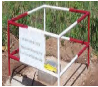
Figure 3: Pillar of the second order RCGN (Republic of Cameroon Geodetic Network) (Carmel, 2012)
