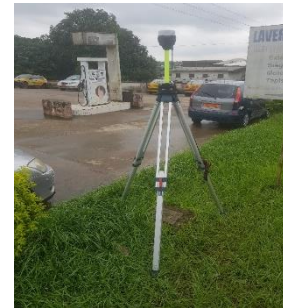
Figure 4: pillar Observe with the rover in dynamic modes (Carmel, 2012)
