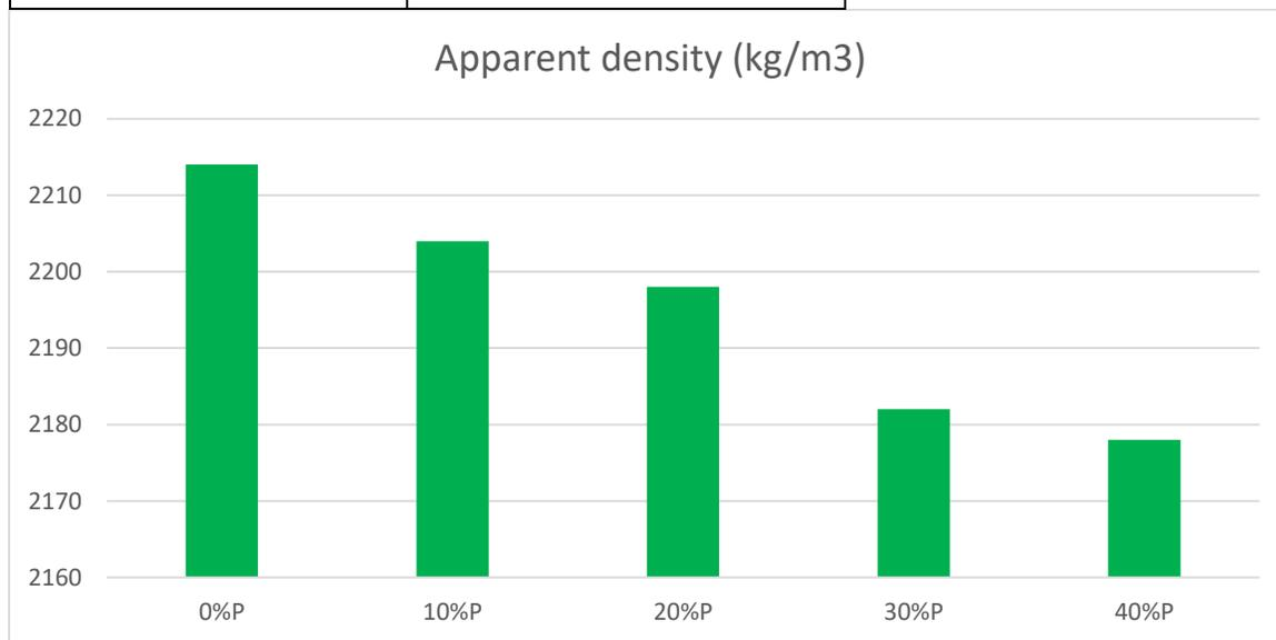
Figure 8: Apparent density of mortars at 28 days.
