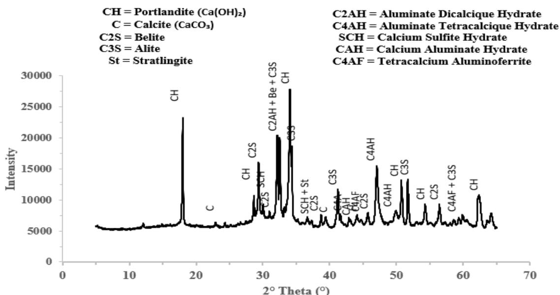
Figure 3: X-ray diffractogram of clinker
