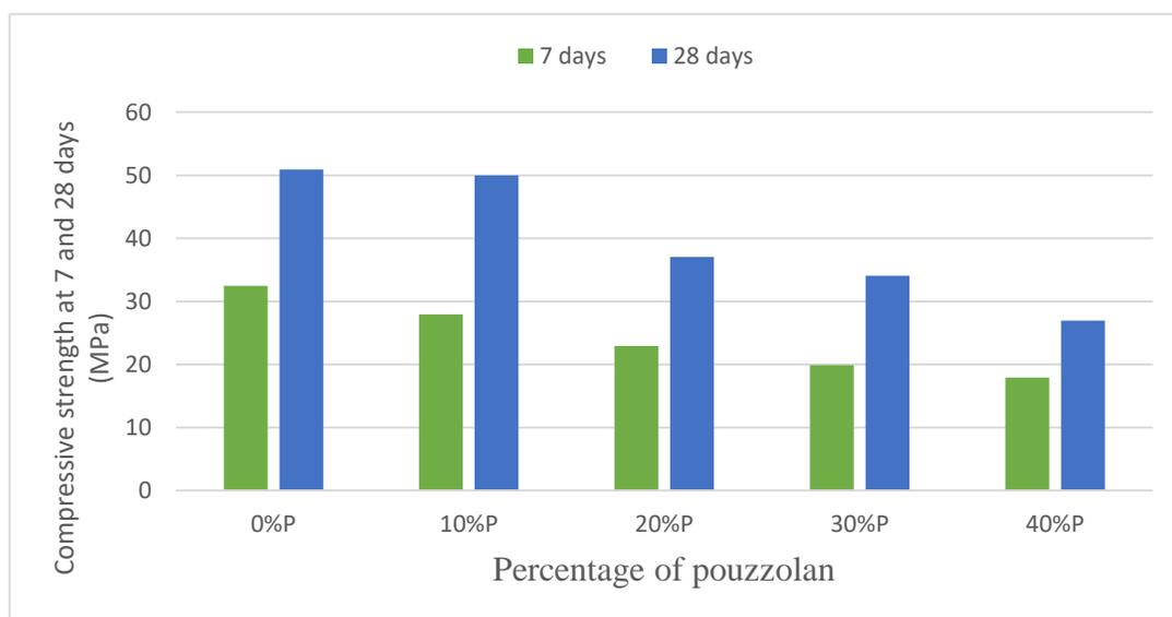
Figure 10: Compressive strength at 7 and 28 days.
