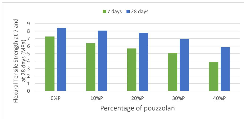
Figure 9: Flexural strength at 7 days and 28 days
