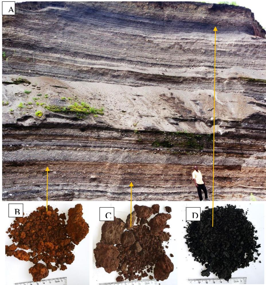
Figure 2: A) Cone of pozzolans in Loum, showing a wide variety of occurrence and colour, B) Red pozzolan, C) Brown Pozzolan D) Black pozzolan
