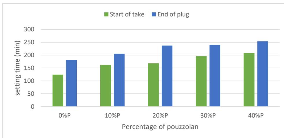
Figure 5: Setting time of the pastes with addition of water
