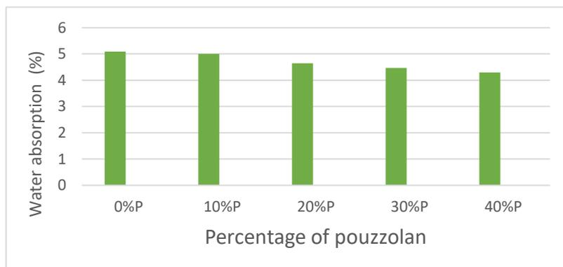
Figure 7: Water absorption of mortars.
