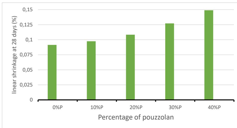
Figure 6: average linear shrinkage of mortars at 28 days
